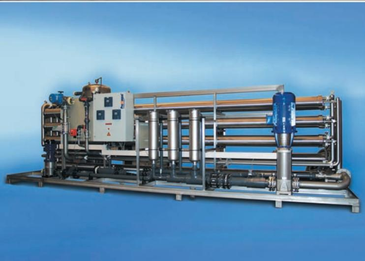
**Reverse Osmosis Systems Dulcosmose® Series BW** are specifically designed for brackish water desalination for drinking water supply as well as for industrial applications. Using state of the art low-pressure membranes, a system salt rejection rate of up to 99 % and a recovery of up to 80 % can be achieved.
