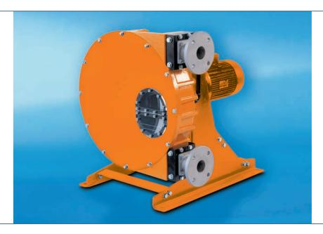
The hose pump DULCO®flex DFDa is designed for largest flow rates and high pressures. It is equipped with pressing shoes and fabric-reinforced hoses. The pump housing is filled with glycerine to reduce friction. A ball-bearing rotor ensures a high level of smoothness and long life. The DFDa delivers flow rates up to 17,500 l/h at backpressures up to 15 bar in tough industrial applications.
