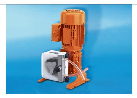
The hose pump DULCO®flex DFAa is designed as low-pressure pump and suitable for use in laboratories as well as OEM applications. It can be used for precise metering of small quantities up to 84 l/h at 2 bar. The rotor is equipped with 3 rollers to reduce pulsation. The hose can be quickly replaced using the quick-release fastener.
