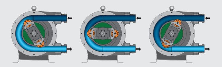
The metering medium is delivered by squeezing the hose with the rotor in flow direction. No valves are required to do so. Abrasive, viscous, and sensitive media are thus gently delivered.
