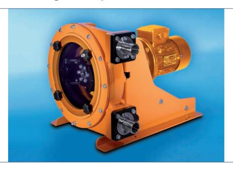
The hose pump DULCO®flex DFCa is equipped with rollers and fabric-reinforced hoses. The DFCa is suitable for tough industrial applications and flow rates up to 12,000 l/h at 8 bar backpressure.
