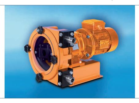
The hose pump DULCO®flex DFBa is designed for small and medium flow rates up to 375 l/h at 8 bar. With rollers and fabric-reinforced hoses, it is suitable for use in tough industrial applications.
