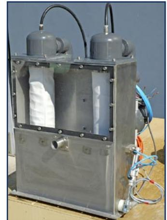
As the powder enters the larger volume of the filtration unit velocity drops and the powder falls to the bottom of the unit. The air is then drawn past the 2 filters, to remove any airborne powder.
